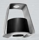
**HD** hangers perform the best when used on equipment located adjacent to stiff support walls and columns, and suspended from narrow rigid upper building spans and used mostly on non-critical vibration sensitive areas.
